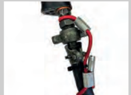
Permanent fixing of the AIRBLOCK between the hose under pressure and the equipment.
