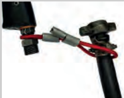
Fixing of the second end of the AIRBLOCK at the hose.
