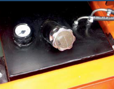
Fuel tank with level gauge
