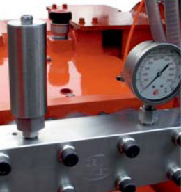
Stainless steel pump-head. Integrated cooling for plunger-seals.
