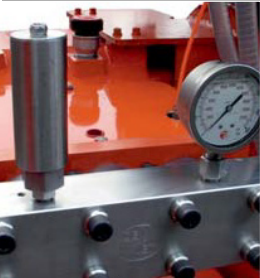
Stainless steel pump-head. Integrated cooling for plunger-seals.
