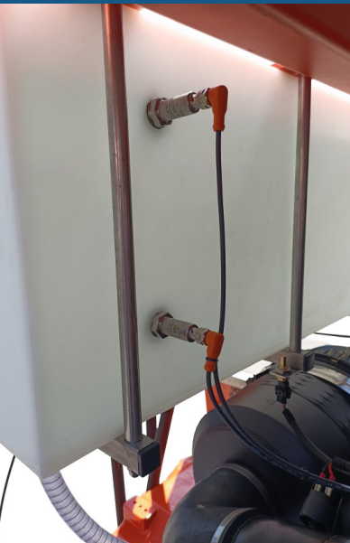
Water level switches
