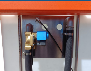
Solenoid valve for water supply
